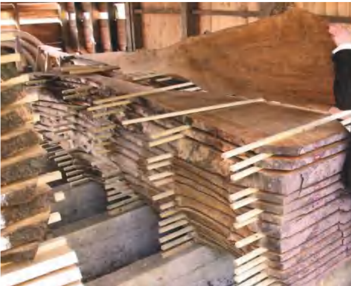
▲ Pic.11 Inside a drying shed or kiln, strips of wood or plastic are laid between the boards to separate them
